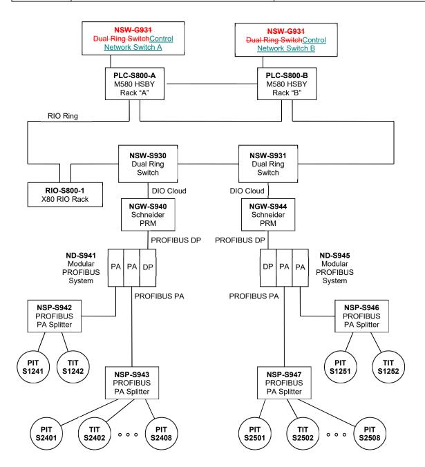
Figure 3-7: Connection of PROFIBUS PA Devices
