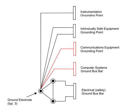
Figure 20-1: Typical Grounding System Implementation with Three Grounding Electrodes *Notes:*
