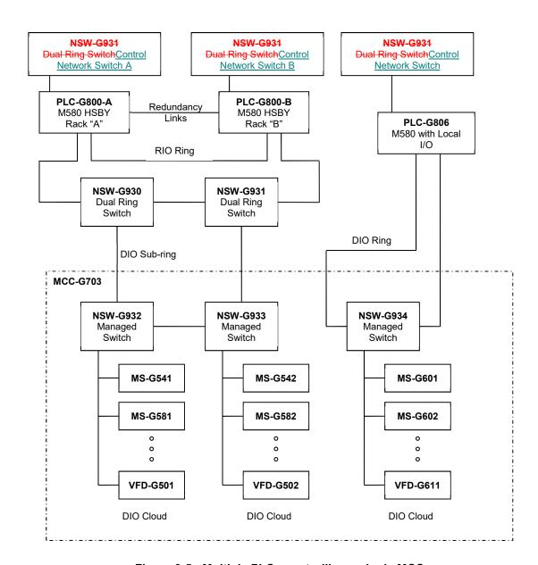
Figure 3-5: Multiple PLCs controlling a single MCC
