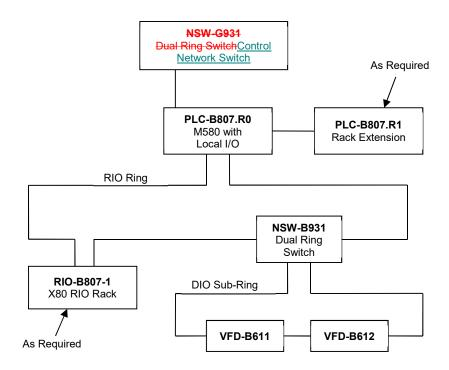
Figure 3-4: Standalone PLC System Architecture with M580 Processor
