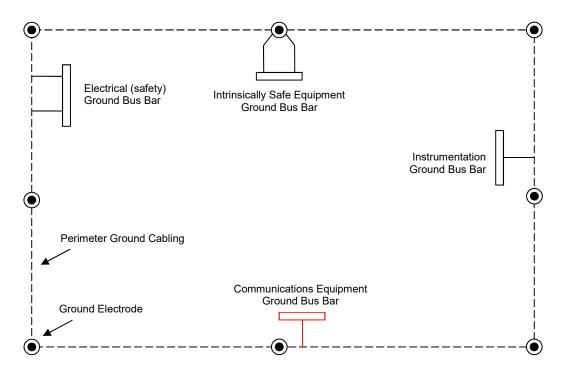
Figure 20-2: Typical Grounding System Implementation with a Perimeter Ground
