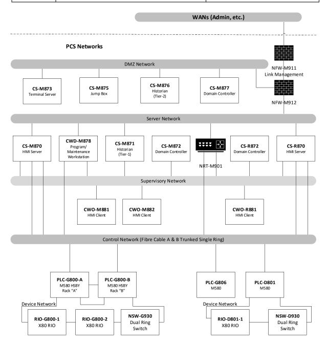
Figure 3-1: Facility PLC-based Process Control System Architecture
